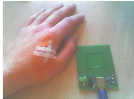
Figure 1: Left hand with EM4102 implant and USB reader
